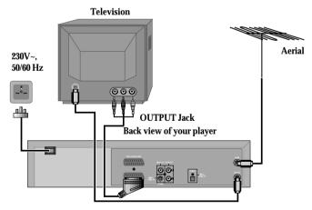
With this connection, if your player is receiving CH BBC1 and your TV is displaying CH3, when you press the [TV/VCR] button on the remote control, your TV will automatically display the CH BBC1. "VCR" will be shown in the display.
